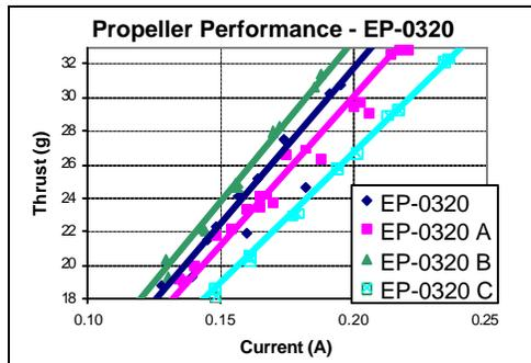
Figure 7 - EP-0320 tip shape testing with RE-16 motor
