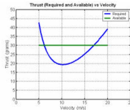
**Figure 3 - Flight velocity envelope with 30 g thrust**
