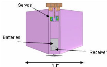
**Figure 10 - Component placement in body**
