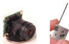
**Figure 8 - Panasonic CX161 camera and BlackWidowAV 2.4GHz Tx**
