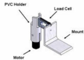
Figure 5 - Static thrust testing setup
