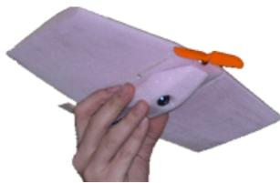
Figure 4 - RIT Thnikkaman MAV (foam construction)
