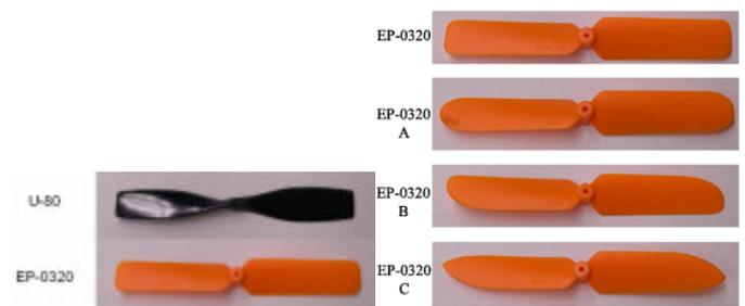
Figure 6 - Propeller tip shapes tested on both U-80 and EP-0320
