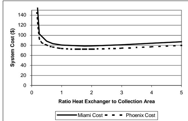
Fig. 4 Cost function for traditional absorber with external shell-and-tube heat exchanger
