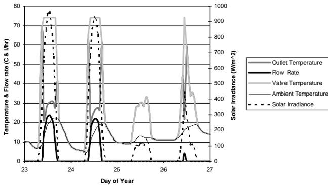
Fig. 3 SPEHX modeled performance for four days in January in Phoenix, AZ.
