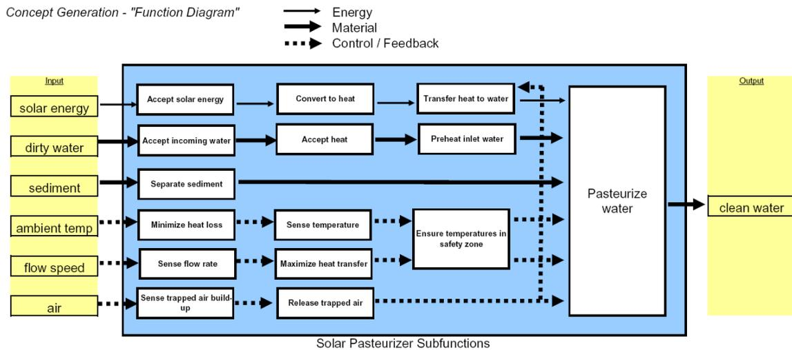
**Figure 3: Energy and Material Function Diagram of Solar Pastuerizer**
