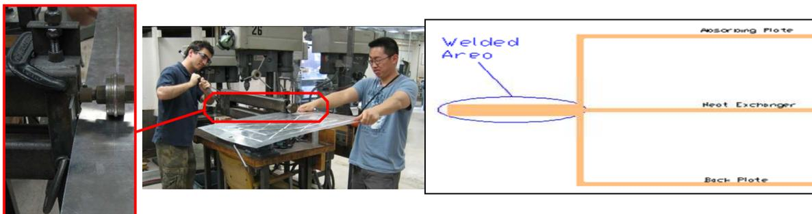
**Figure 7: Simple mechanical crank used to make z-bends on edges and ribs for lateral support. A cross section of the collector and heat exchanger edge using the mechanical crank, which enabled a one weld pass for the entire system.**
