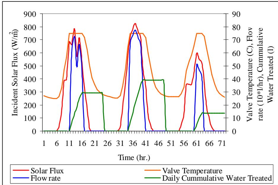
**Figure 6: Three typical days of solar pasteurizer output for a given set of design parameters.**
