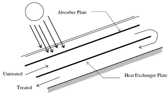
**Figure 1: Schematic of solar pasteurizer with integral heat exchanger.**
