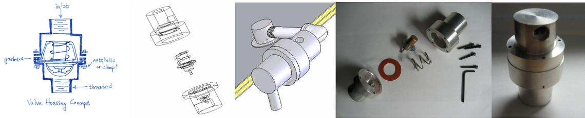
**Figure 3: Concept, final design, and prototype of flow/temperature regulation subsystem.**
