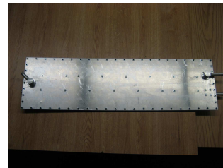
Figure 10: Assembled heat exchanger
