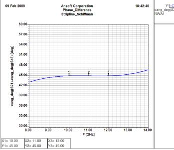
Figure 4: Physical Designer model phase difference, markers showing 45° at 10GHz, 11GHz, and 12GHz.
