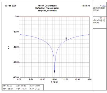
Figure 7: Physical Designer model reflection. Markers at 11GHz (-31.07dB), 12GHz (-73.76dB), and 12GHz (-31.07dB).
