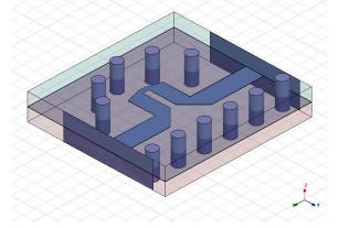
Figure 2: Schiffman phase shifter model in HFSS, with vias.
