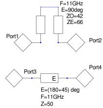
Figure 1: Schematic View of Ideal Schiffman
