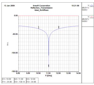
Figure 6: Ideal model reflection. Markers at 11GHz (-34.88dB), 12GHz (-138.14dB), and 12GHz (-34.88dB).
