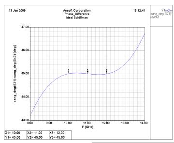
Figure 3: Ideal model phase difference, markers showing 45° at 10GHz, 11GHz, and 12GHz.
