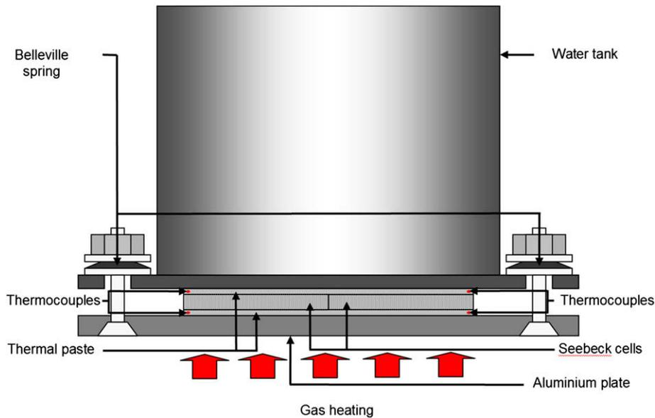
Fig. 12. TE power generator experimental set up.
