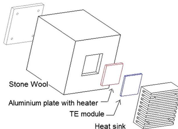
Fig. 3. Experimental TE power generator test system.
