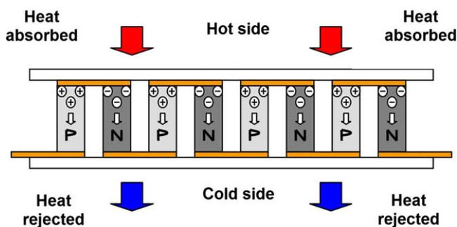
Fig. 2. Working of a Seebeck cell.
