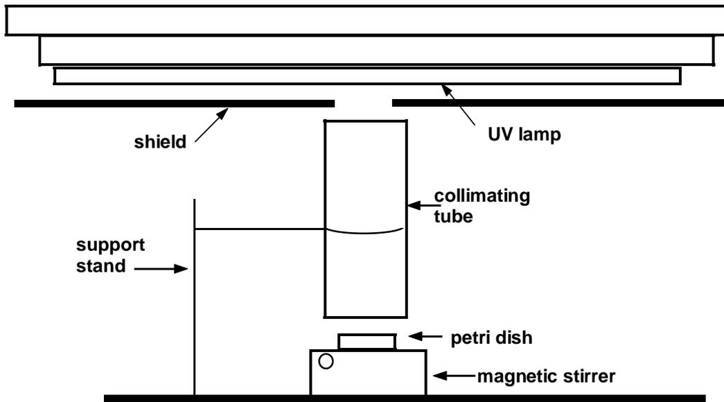
NOTE 1 – The collimating tubes shall be a minimum of 53 cm (21 in) in length and the interior shall be painted flat black.
