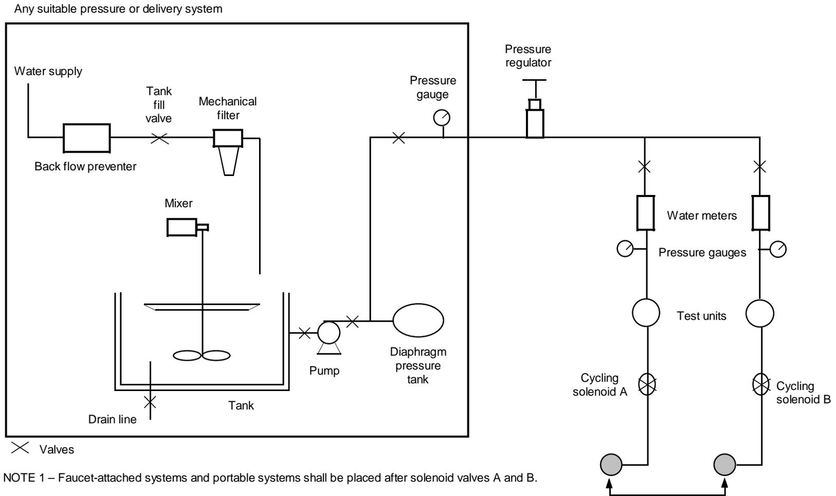
NOTE 1 – Faucet-attached systems and portable systems shall be placed after solenoid valves A and B.
