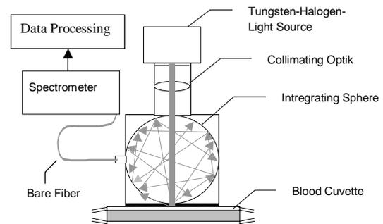
Figure 1: Schematic illustration of a functional model for measuring haematocrit and oxygen saturation in extracorporeal circulation systems.
