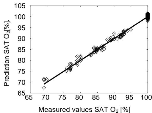
Figure 3: Prediction of oxygen saturation compared to measured values SatO<sub>2</sub>, PRMSE: 0,9 %, n<sub>p</sub>: 4, n<sub>dat</sub>: 150
