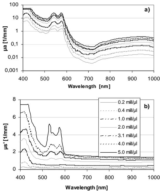
Figure 2: Absorption coefficient (a) and reduced scattering coefficient (b) in the spectral range 400 to 1000 nm for various red blood cell concentrations.
