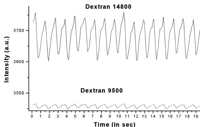
Fig. 6. Pulsatile signals obtained *in vitro*. For high-molecular dextran, the pulsations are much larger.
