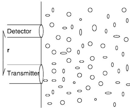
Fig. 3. Geometry of two fibers facing a half-space blood medium perpendicularly.
