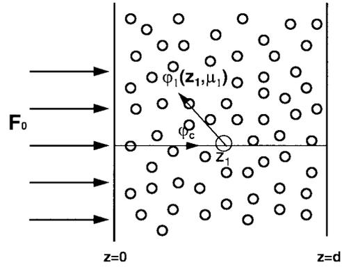
Fig. 1. Definition of first-order scattering in successive order scattering transport approximation.
