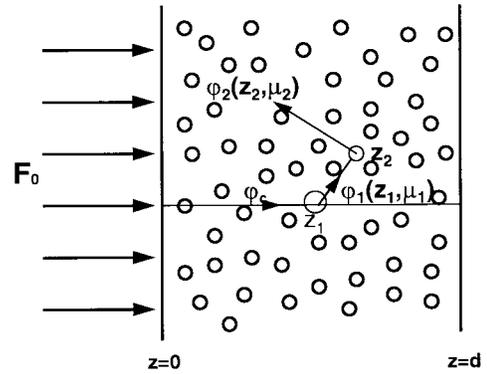
Fig. 2. Definition of second-order scattering in successive order scattering transport approximation.
