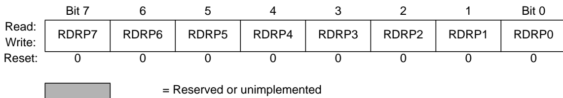
Figure 3-25 Port P Reduced Drive Register (RDRP)
