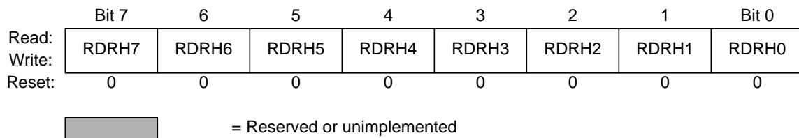
Figure 3-33 Port H Reduced Drive Register (RDRH)
