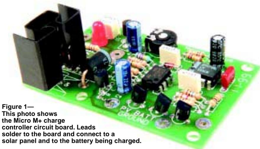
Figure 1— This photo shows the Micro M+ charge controller circuit board. Leads solder to the board and connect to a solar panel and to the battery being charged.
