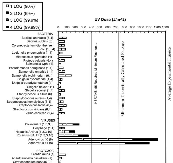
**Figure 4: Log inactivation of pathogens based on theoretical and experimental fluence [10].**
