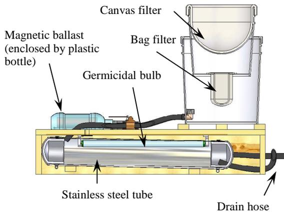
**Figure 7: Section view of the UV Tube**
