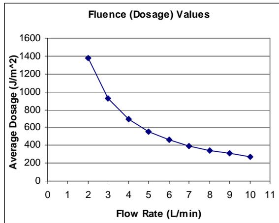
**Figure 3: Conservative model of UV dosage at varying flow rates**
