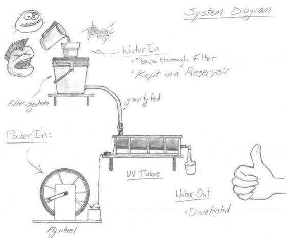
**Figure 1: Final system concept**
