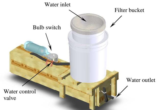
**Figure 6: The UV Tube final design**
