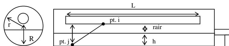
**Figure 2: Definition of variables for irradiance model**
