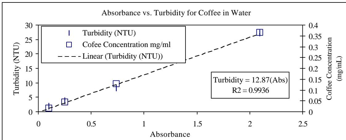
Note: Measurements were performed by Sarah Brownell in August 2001, using Folgers® Classic Roast Coffee Crystals and a Pharmacia Ultraspec® III UV/Visible Spectrophotometer and a Hach Pocket Turbimeter™.
