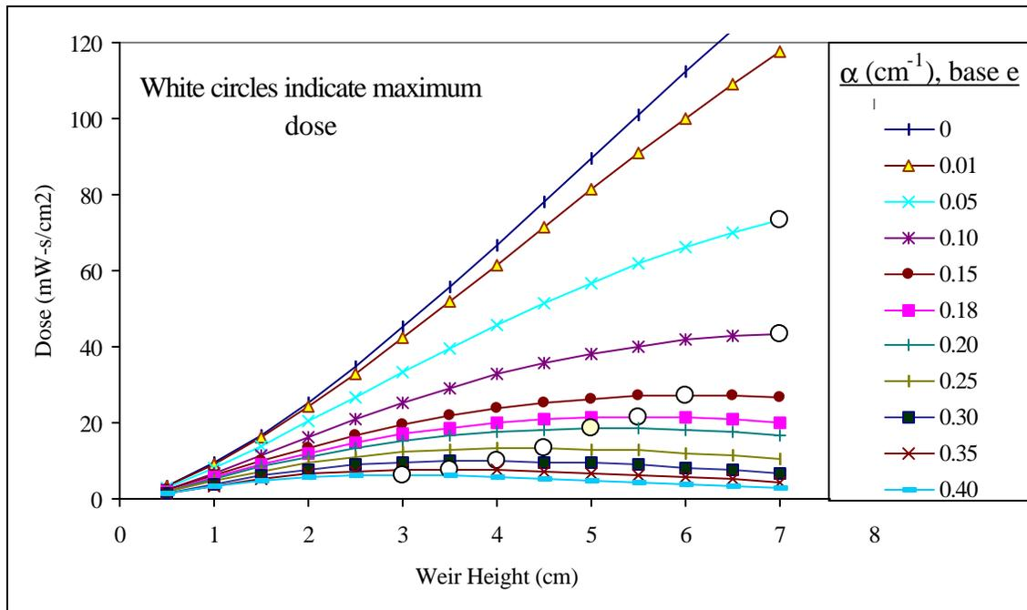
Note: White circles indicate maximum dose for each absorption. Data are from PSS Model output, described in section VII beginning on page 45. Code input for Engineering Equation Solver (EES) used to compile the above predictions can be found in Appendix A.
