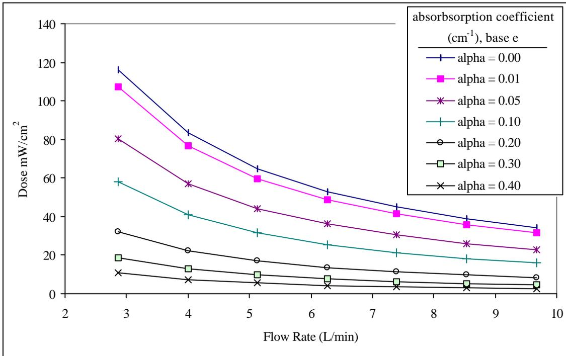
As can be seen in Figure 30, the dose decreases rapidly as flow rate increases for small alpha values. As the absorption coefficient increases the change in dose for increasing flow rate decreases. Therefore, for water with a high absorption coefficient, decreasing the flow rate will not increase the dose by very much. This pattern is one reason why knowing the absorption coefficient is so critical to predicting performance.
