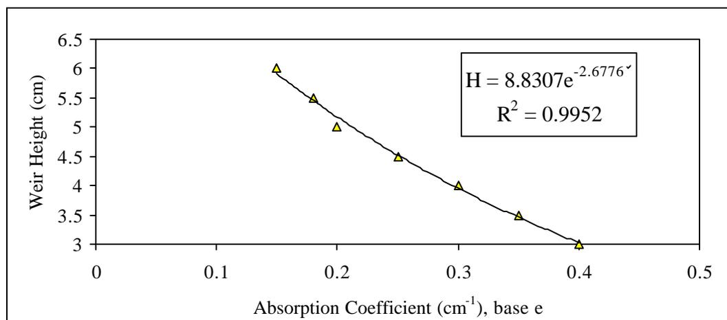
Initially a weir height of 4 cm was used. Based on the above predictions, and expected absorption coefficients less than 0.20, an even higher weir height might be recommended. However, the design is limited by the overall diameter of the tube. Due to additional water that accumulates over the weir height during flow (about 0.6 cm for 5 L/min flow, for further discussion see page 48) and the 4-5 cm that the bulb takes up, a 4 centimeter weir is maximum height without risking bulb wetting.
