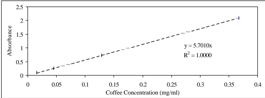
Note: Measurements were performed by Sarah Brownell in August 2001, using Folgers® Classic Roast Coffee Crystals and a Pharmacia Ultraspec® III UV/Visible Spectrophotometer.
