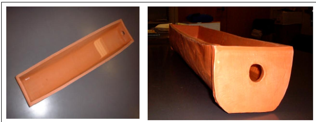
After firing the pottery UV-Tube, nicknamed the “UV-Trough”, it was filled with water. Capillary action was observed and the outside had begun to sweat within the first twenty minutes. After a couple of hours the volume of water had been reduced substantially and there was a small puddle underneath the UV-Trough, presumably where evaporation had not been possible. The piece was placed under UV light for five days, after which time no iron was detected in the water.
