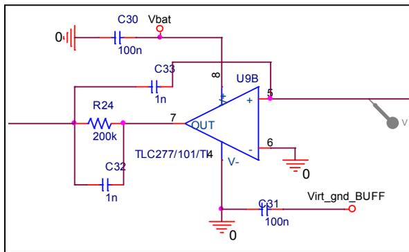
Figure 9: Right Leg Drive Circuit
