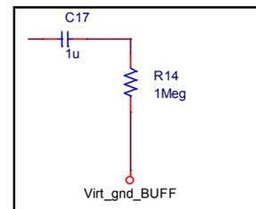
**Figure 6: One of two Passive High Pass Filters used to define the lower cutoff frequency of the amplifier**
