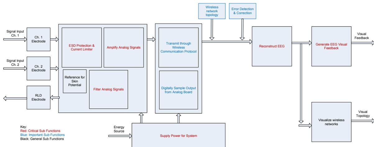
Figure 1: System Level Block Diagram of the Wireless EEG System
