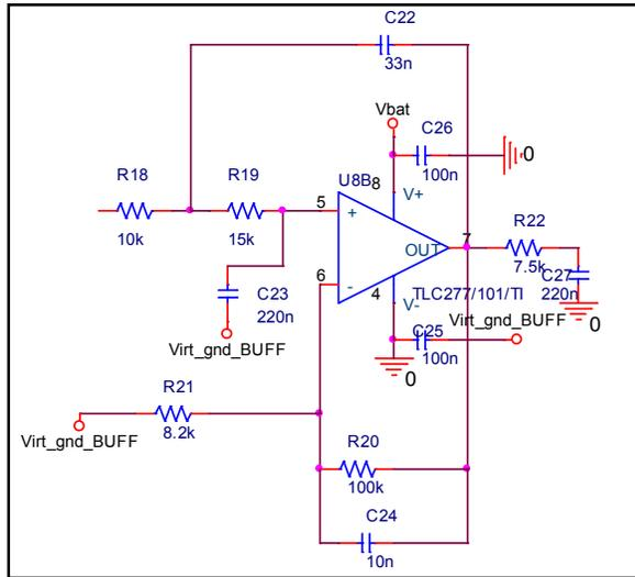
Figure 8: 3rd Order Low Pass Bessel Filter Stage implemented using the TLC 277 operational amplifier
