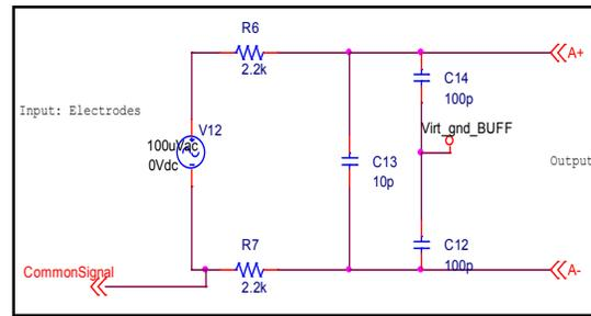
**Figure 4: High Frequency Rejection Circuit with its output going to the Instrumentation Amplifier Stage through an ESD Protection Diode**
