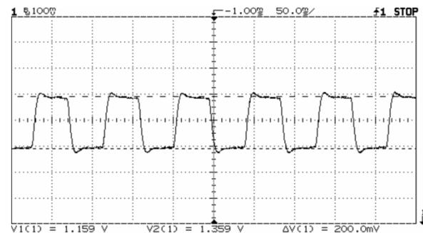
**Figure 13: Square Wave Calibration Test Output**
