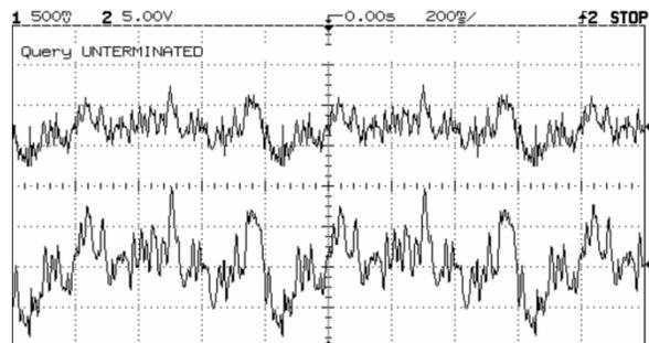
**Figure 15: Sample EEG input signal (Top) and the processed output signal (Bottom) from the amplifier. Note that the input signal is divided by a factor of 10000 using a voltage divider before being applied to the amplifier.**
