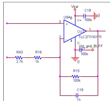
**Figure 7: Adjustable Gain Stage implemented using the TLC277 operation amplifier**
