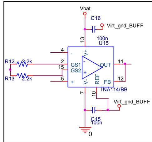
**Figure 5: Instrumentation Amplifier Stage implemented using the INA114 amplifier**
