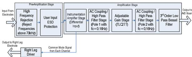
**Figure 3: System Level Block Diagram for the Analog Board**
