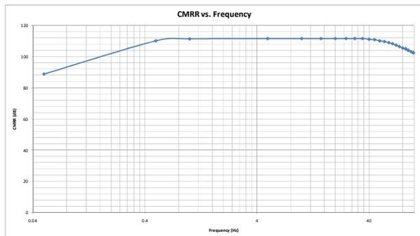
**Figure 15: CMRR Vs Frequency for the EEG Amplifier**
