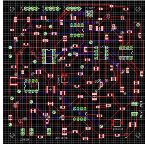
Figure 10: Trace Diagram for the Analog Board Design
