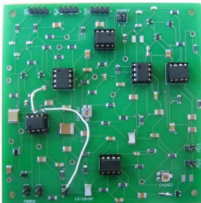
**Figure 12: Completed Analog EEG Board**
