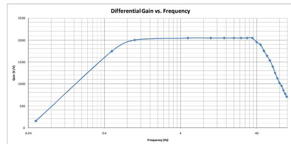
**Figure 14: Differential Gain Vs. Frequency Plot for the EEG Amplifier**
