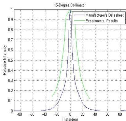
Figure 1: Light distribution curve for 15-Degree Collimating Lens
