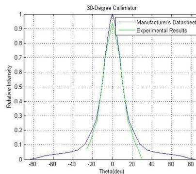
Figure 2: Light distribution curve for 30-Degree Collimating Lens
