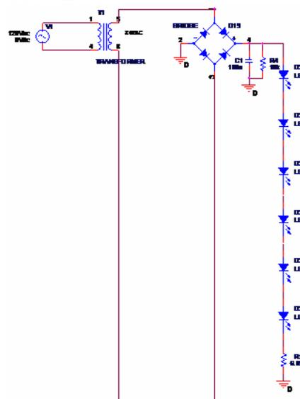
Figure 8: Single LED board schematic
