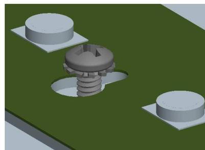
Figure 5: Keyhole PCB Attachment
