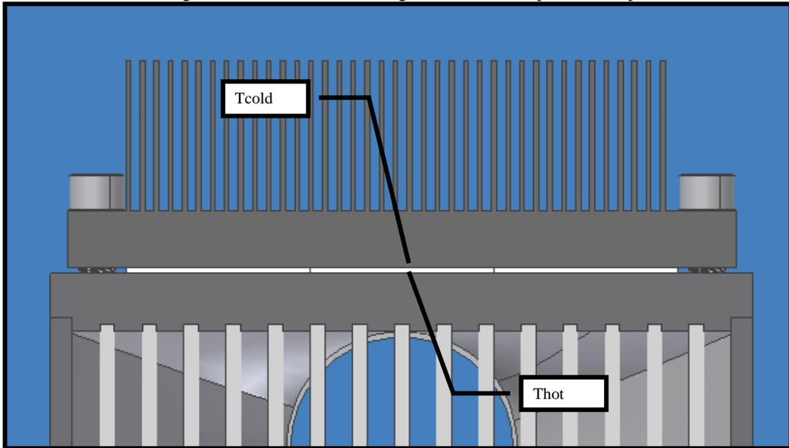
The temperatures at the inlet and exit are needed for the system efficiency calculations. These thermocouples are built into the test stand.
