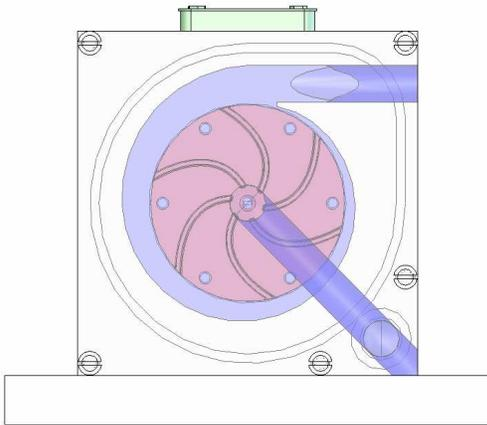
**Figure 1: Front view of the housing showing the volute (light blue), and the interfering inlet (dark blue).**
