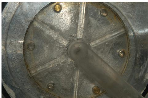
**Figure 3: View of optically clear pump housing (at 1700 rpm) and results that can be achieved with a high speed camera**
