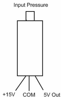
Figure 3: Wiring Diagram of PX-209
