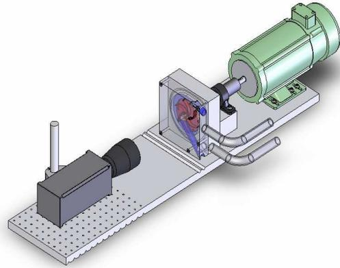
**Figure 2: View of the pump subsystem showing the camera, housing, and motor.**
