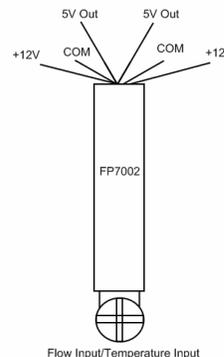
Figure 4: Wiring Diagram of FP7002
