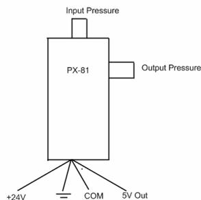
Figure 4: Wiring Diagram on PX-81
