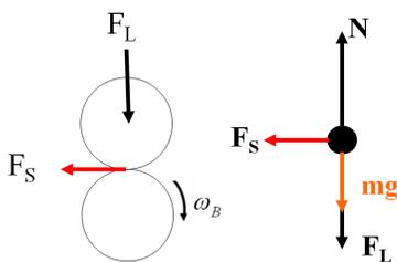
Figure 7: Illustration of interaction of forces between the top and bottom roller
