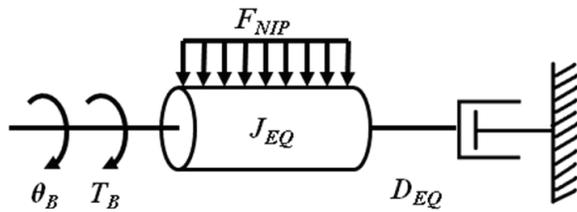
Figure 6: Physical representation of bottom model
