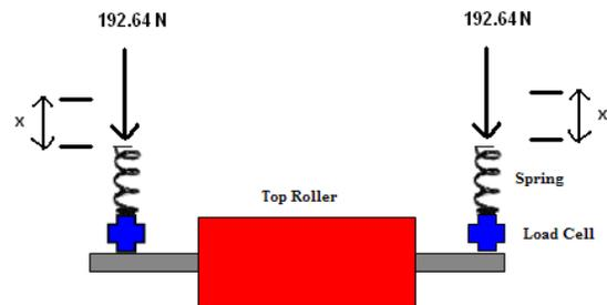
Figure 11: Description of dividing the force between the two springs
