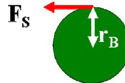
Figure 9: Visual representation of relationship between bottom roll torque, radius and frictional force (F<sub>S</sub>)
