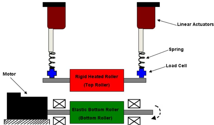
Figure 1: Roller Fuser Test Bed (RFTB)
