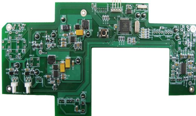
**Figure 5: Completed PCB with Subsystems Populated**
