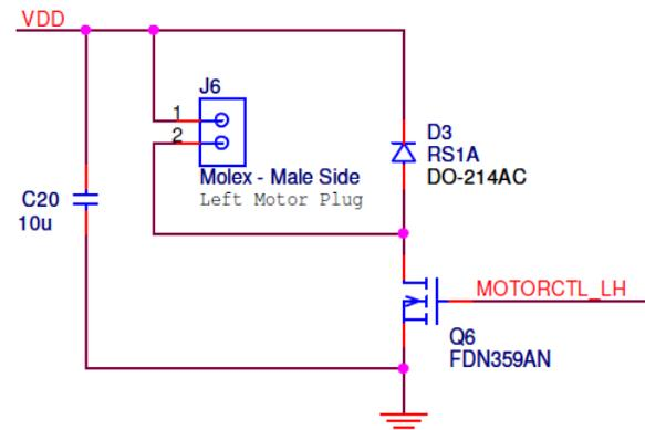
Figure 3 - Motor Driver Circuit
