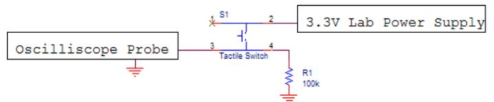
Figure 2 - Switch Bounce Measurement
