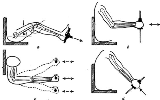
**Figure 4 - Diagram demonstrating the different orientations of how a seated force could be applied**
