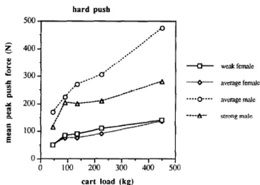
**Figure 9 – Mean Peak hard push force on cart handles based on load (Chaffin and Resnick, 1995)**
