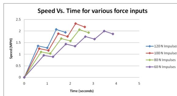
**Figure 7 – Relationship between time to reach a maximum speed at different applied forces**
