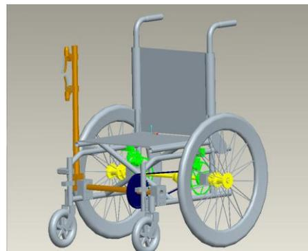
Figure 3 – Lever Differential Model
