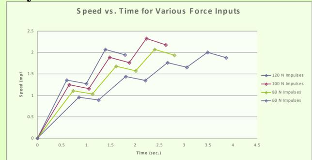
The chart above displays the time required to achieve a speed of just under 2 mph for various inputs of force. Each peak denotes a power pulse or a round-trip movement of the lever. The chart shows that the lower the amount of force applied the longer it takes to achieve a desired speed.
