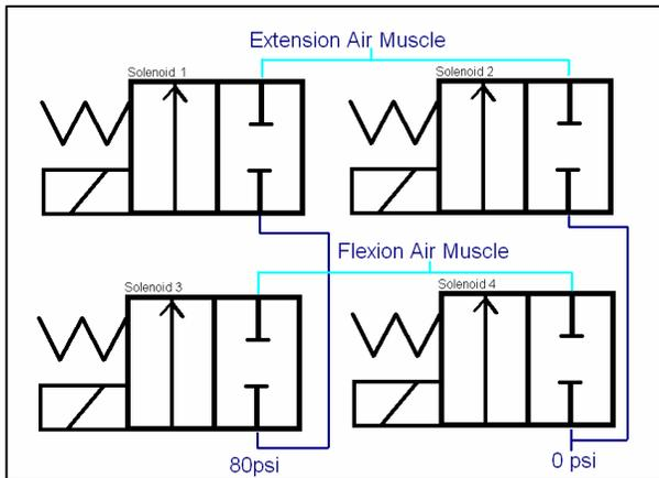
**Figure 1 - Four 2-Position, 2-Way Solenoids for 1 DOF**
