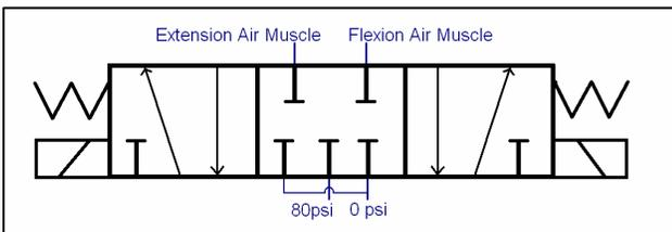
**Figure 2 - 3-Position, 4-Way Solenoid for 1 DOF**
