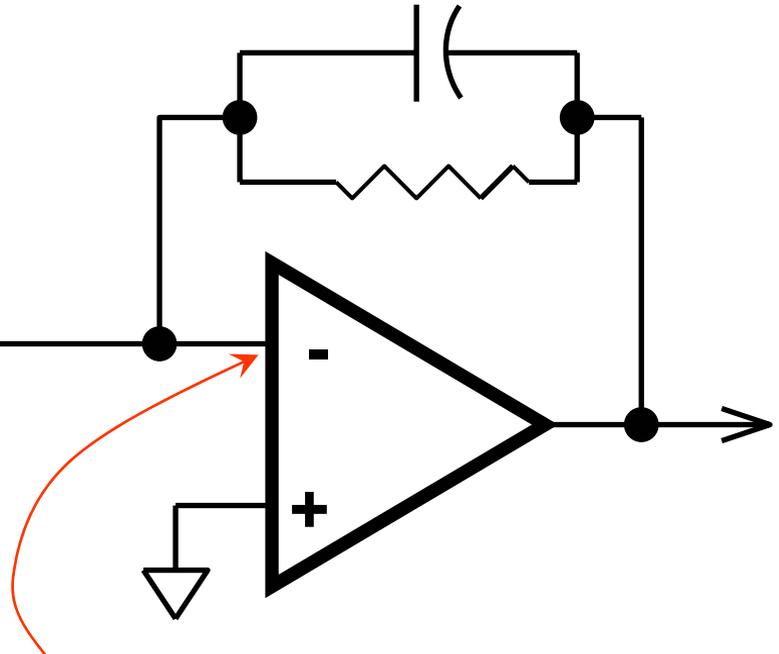
**Input pins will have small currents in or out of the pin (bias current).**
