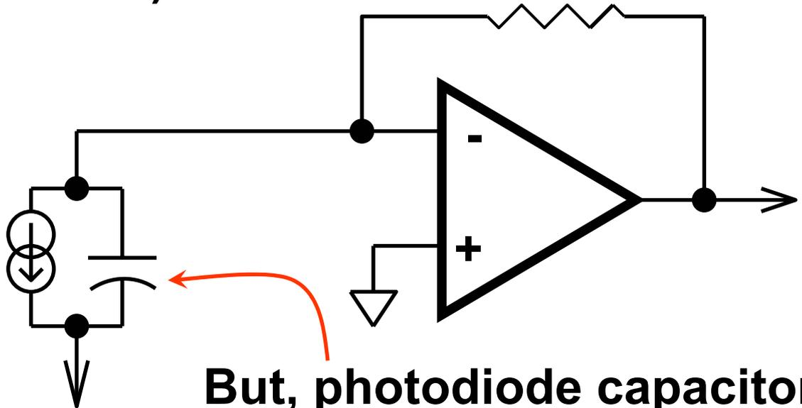
**But, photodiode capacitor means feedback signal will lag the actual output change.**
