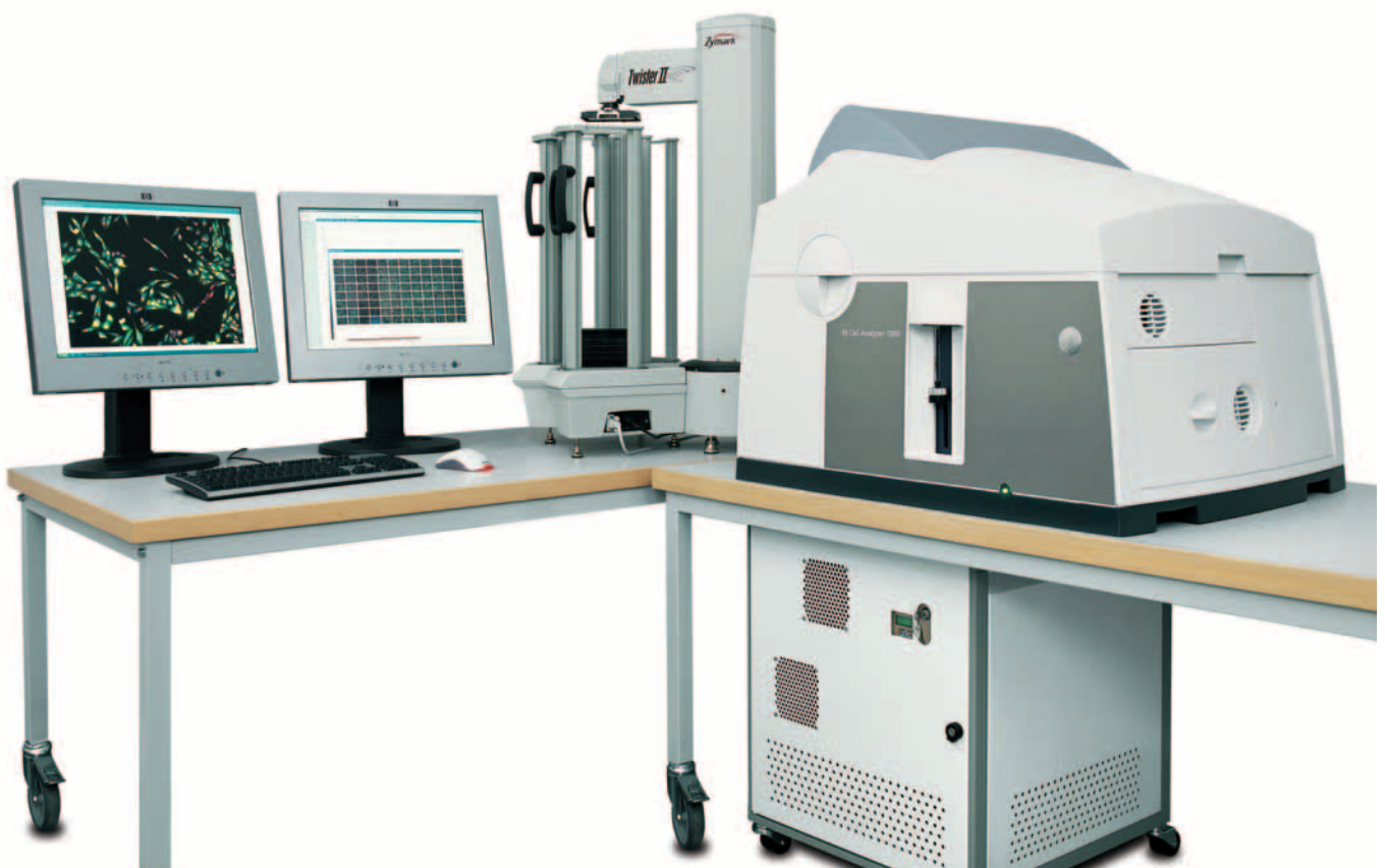
Fig 1. IN Cell Analyzer 1000 is a modular and fast analysis platform for cell-based assays.
