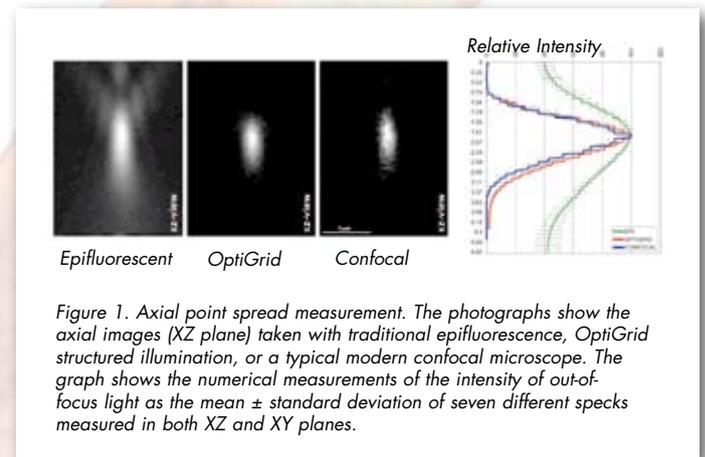
Figure 1. Axial point spread measurement. The photographs show the axial images (XZ plane) taken with traditional epifluorescence, OptiGrid structured illumination, or a typical modern confocal microscope. The graph shows the numerical measurements of the intensity of out-of-focus light as the mean  $\pm$  standard deviation of seven different specks measured in both XZ and XY planes.
