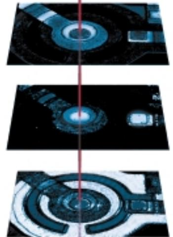
OptiGrid's research-quality digitized optical sections allow full-focus digital compilations and 3-D digital projections.
