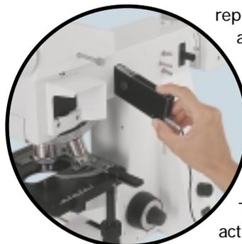
With the slider module inserted, you can view confocal images on your computer monitor. With the OptiGrid slider module removed, your microscope and camera will function normally.
