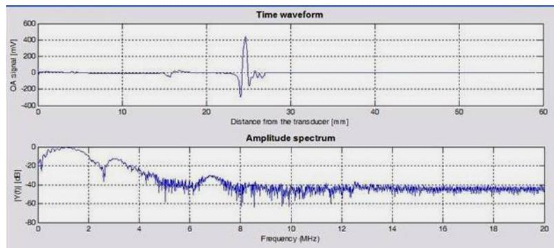
**Figure 3:** Sample A-line trace and corresponding frequency spectrum from 1mm tube with cupric sulfate.
