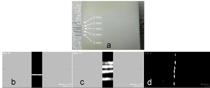
**Figure 2.** Picture of plastisol phantom with six horse hairs separated by varying distances (a). Axial slice shows top horse hair in long axis (b). Coronal slice shows 4 hairs in long axis (c). Sagittal slice shows all six hairs in short axis (d).
