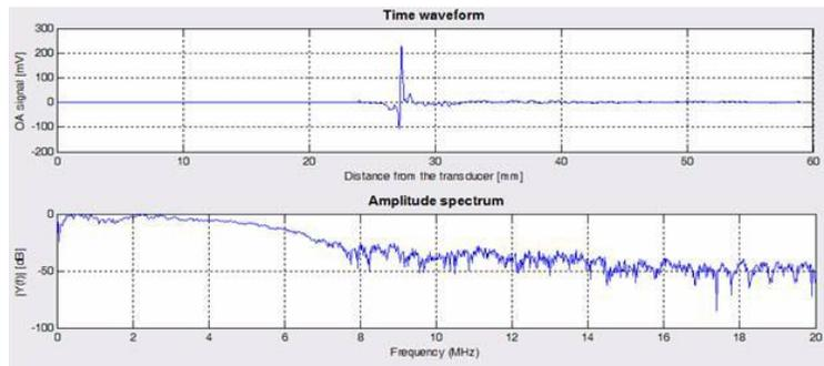
**Figure 1:** Plots showing typical A-line response from single horse hair and the corresponding frequency spectrum.
