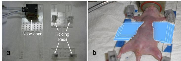
**Figure 5.** Picture showing two specimen holders with the nose cone and holding pegs (a). Final mouse configuration (b).
