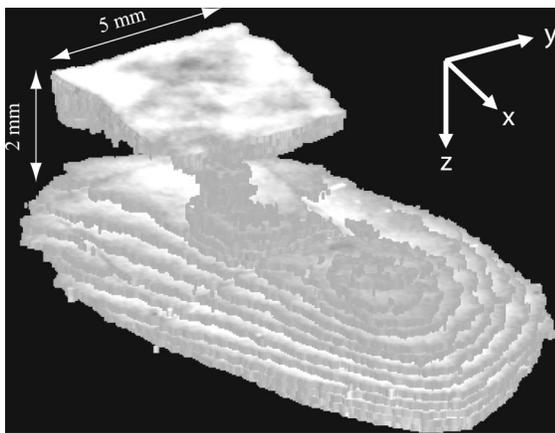
Fig. 5. Optical tomograph of the heterogeneous turbid phantom from frequency-derivative images.
