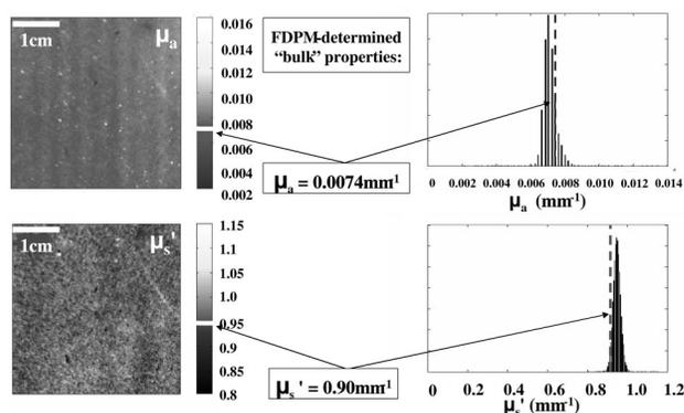
Fig. 2. Absorption (top) and scattering (bottom) data of the spatially varying phantom optical properties. Quantitative images (inverse millimeters, left) and corresponding pixel histograms (right) demonstrate good agreement with known bulk properties.
