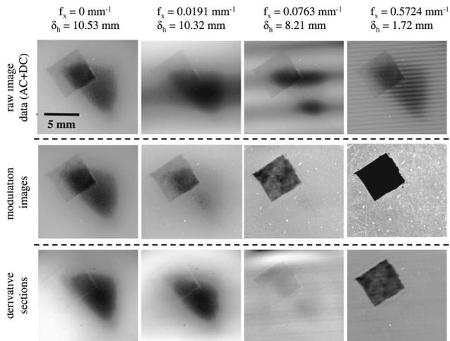
Fig. 4. Top to bottom, raw reflectance, ac modulation, and frequency-derivative images of the heterogeneous phantom.
