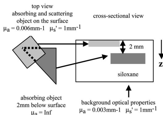
Fig. 3. Schematic diagram of a heterogeneous phantom.
