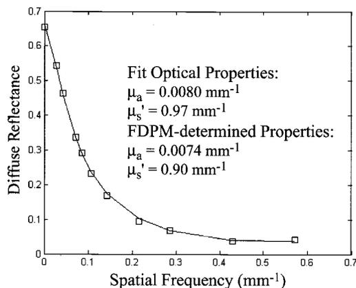
Fig. 1. Example multifrequency data (open squares) and corresponding fit (solid curve). The turbid medium acts as a low-pass filter.
