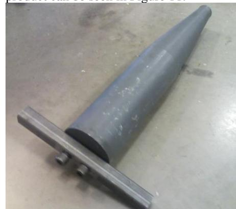
Figure 11: The body mold fixture with the wing attachment.
