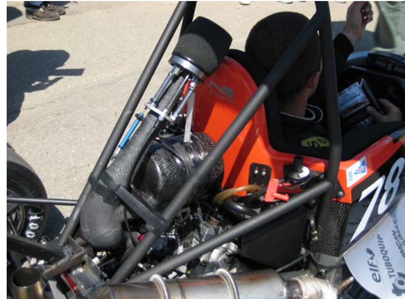
Above: Partial Monocoque Roll Hoop Mounting (ETS)
