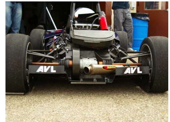
Above: Diffuser Tunnels (TU Graz)
