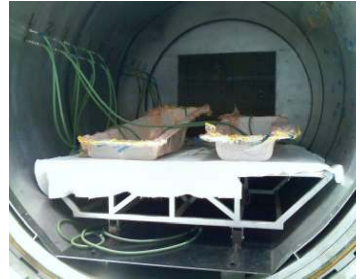
Autoclave Cure of Components (CSU Northridge)
