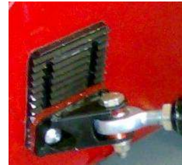
Composite Tab Bolted to Chassis (RMIT)
