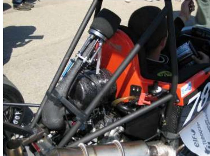
Above: Partial Monocoque Roll Hoop Mounting (ETS)
