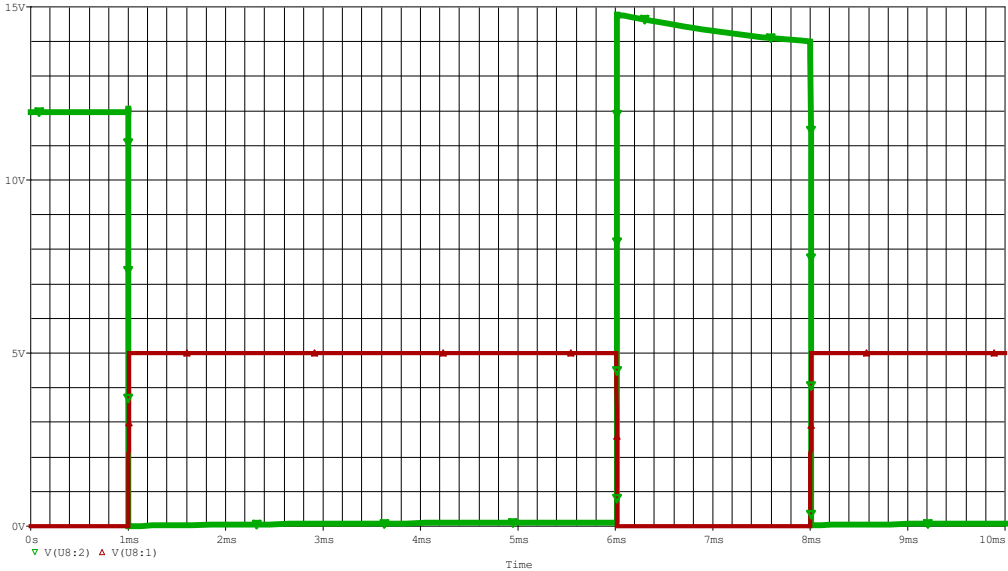
Figure 2: Injector Simulation Output Voltages with Implementation of Injector Feedback Diode
