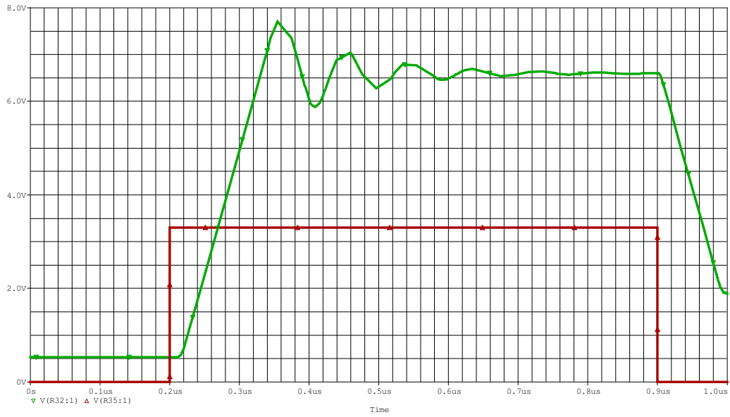
Figure 20: Simulation Voltage Outputs for Original ECU Relay Control Scheme
