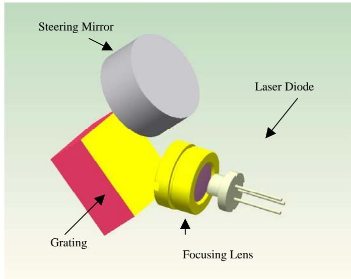
Figure 2. The tunable laser system consists of a 785 nm laser diode that is coupled into an external cavity consisting of a focusing lens and a grating. The first diffraction order of the grating is directed back into the laser diode while the zero order is directed to a steering mirror.
