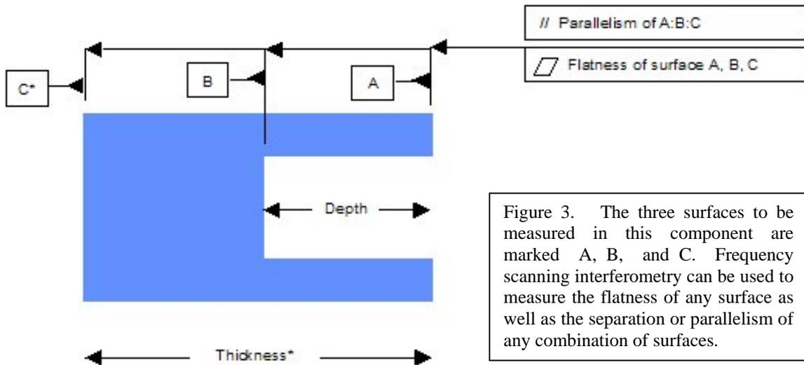
Figure 3. The three surfaces to be measured in this component are marked A, B, and C. Frequency scanning interferometry can be used to measure the flatness of any surface as well as the separation or parallelism of any combination of surfaces.
