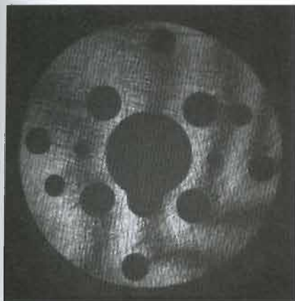
Figure 2. An interferogram of a spacer used in a fuel injector application displays dark and light bands — interferometric fringes that show the deviation from an ideal plane.
