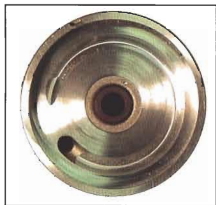
Figure 8. Proper operation of today's automotive fuel pumps requires tight control of the flatness, parallelism and height between the outer ring and the recessed surface of the impeller housing.
