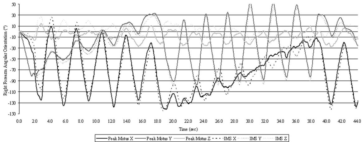
**Fig. 3 Angular orientation in three dimensions of the forearm performing a back and forth, up and down sweeping motions in the forward reach space envelope of the subject**
