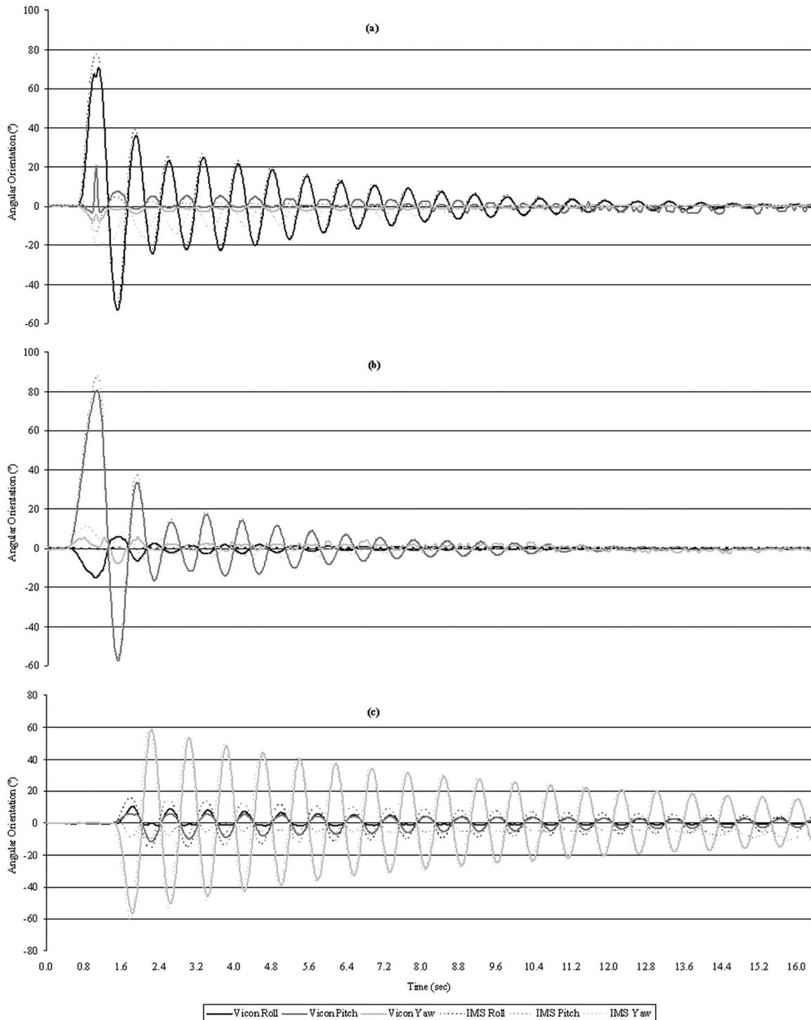
**Fig. 2 Angular orientation time series from gold-standard Vicon estimate versus IMS during pendulum motion occurring about dominant axis of (a) roll axis, (b) pitch axis, and (c) yaw axis**
