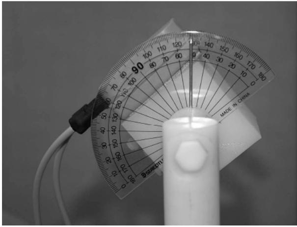
**Fig. 1 IMS setup for static testing. Sensor is attached to rotating white block and rotated while the metal pointer indicated the orientation estimate on the protractor.**
