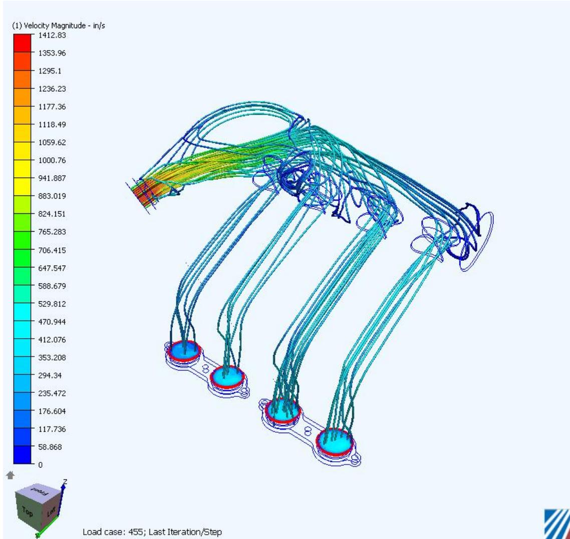
CFD will be used to compare our design iterations and to select an optimized geometry.
