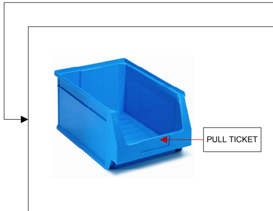
Picker puts pull ticket in bin pocket after part has been picked.
