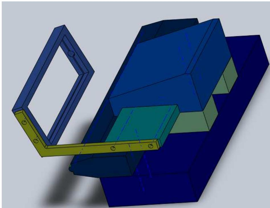
6. 30 degree angle blocks and paper spooling device. (this angle may differ depending on the device used. This angle was chosen so that by tipping the device forward the camera would not be looking at any of the components underneath the spool.)
