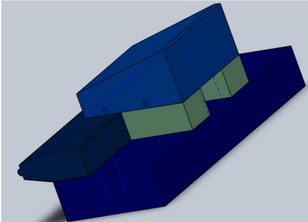
**Figure:** base block, fiber optic bar, 2 spacing blocks and 15 degree angle block all attached together.
