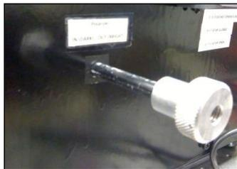
Move polarizer pull lever to the fully extended position so that all light is passing through it. There are two positions for the sliding polarizer to get the “bright” or “dark” image. Pulling the rod outward will be the “bright” position.
