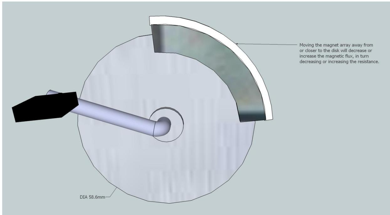
We plan to reuse the current adjustment knob on the friction system to raise and lower the magnet array. This will increase and decrease the flux, and in turn affect the difficulty of pedaling in the same way. With the fine adjustment, the PT should be able to accommodate a wide range of abilities.
