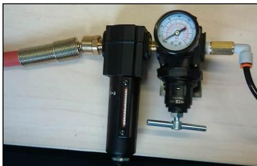
Figure 9 - Filter and Regulator Setup
