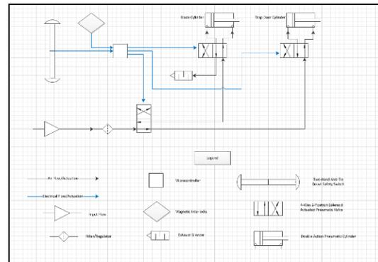
Figure 4 - Original Pneumatic System
