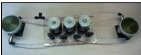
Figure 7 - Two Handed Anti-Tie Down Setup
