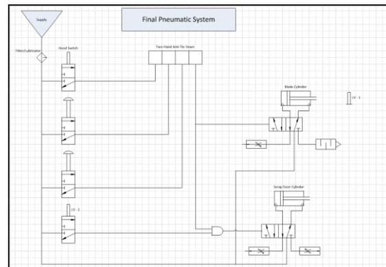
Figure 5 - Final Pneumatic System
