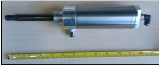
Figure 6 - Cylinder to Actuate Cutting Blade Carriage
