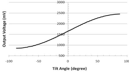
Fig. 4. Nonlinear relationship output of x-axis accelerometer.
