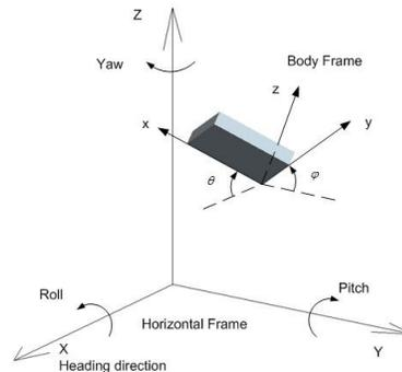
Fig. 3. Coordinate frames (body frame and horizontal frame).
