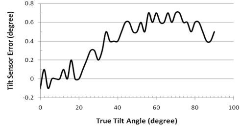
Fig. 5. Tilt errors due to the nonlinear characteristics of the accelerometer (average error: 0.38°).
