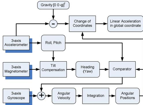
Fig. 1. Complementary filter approach to the inertial/magnetic tracker.
