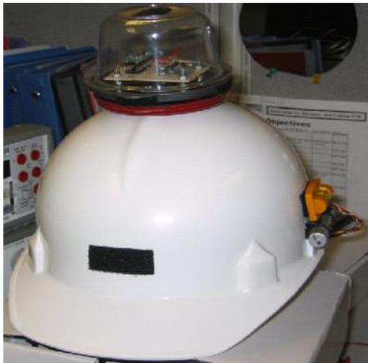
Fig. 3: ECROM system mounted on a hard hat
