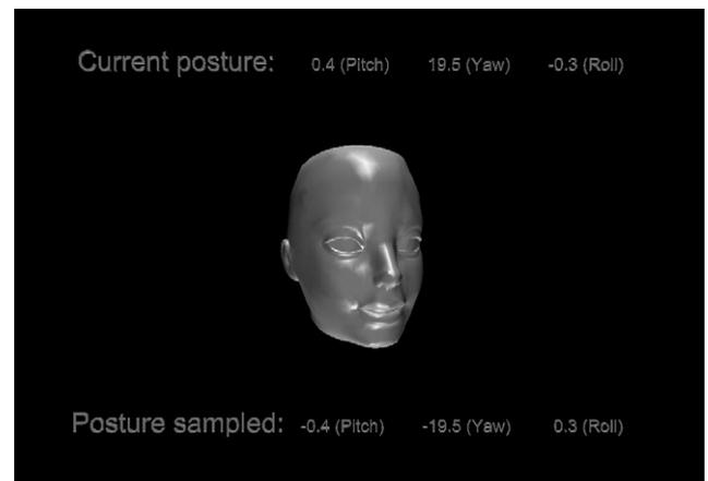
**FIGURE 2.** Screen shot of digital head posture measuring device's display of simulated head movements and numerical outputs. Current posture values change in real time, and posture can be sampled and recorded at any time by the user. The abnormal head posture depicted has a chin up of 0.4 degrees, head turn of 19.5 degrees to the right, and head tilt of 0.3 degrees to the left.
