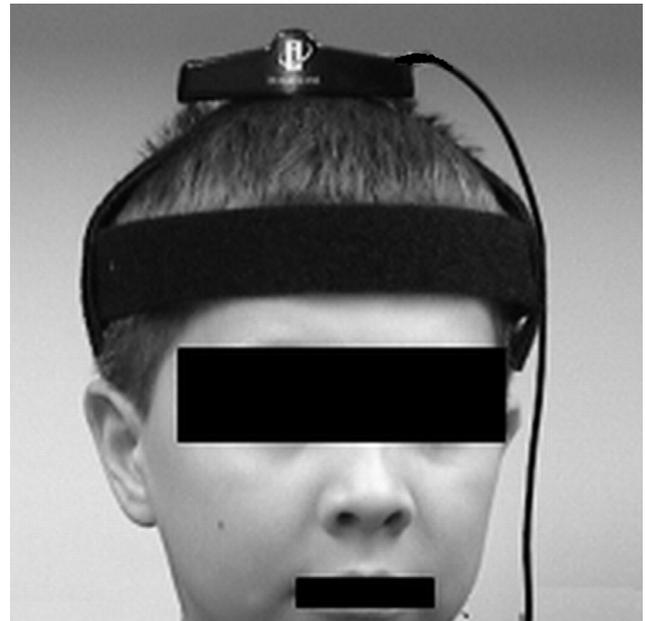
**FIGURE 1.** Photograph showing the modified digital head posture measuring device with 2 Velcro strips (Velcro Brand Fasteners, Clifton, New Jersey, USA) and a motion tracker mounted on a child's head. The black cord leads to a USB connection that is inserted into the computer used to record subject head postures.
