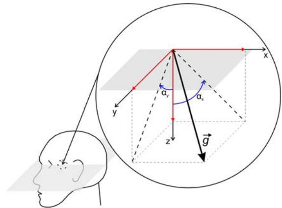
Fig. 1 Head tilt sensing with a triple axis accelerometer
