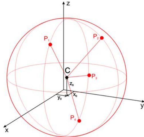
Fig. 2 Calculating accelerometer offset corrections with the equation of a sphere from 4 points.
