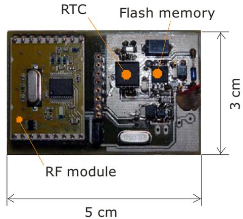
Fig. 4 Top side of the printed circuit board of a prototype device.
