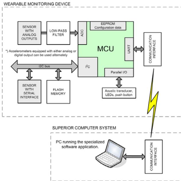
Fig. 3 A block diagram of the designed device
