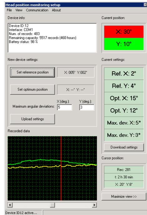
Fig. 5 A screenshot of a computer software application used for setting up the device and data acquisition.
