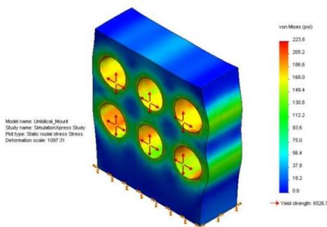
Figure [6]: Stress/Deformation simulation in CAD
