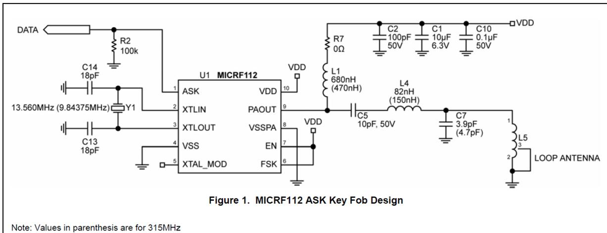
Figure 1. MICRF112 ASK Key Fob Design
