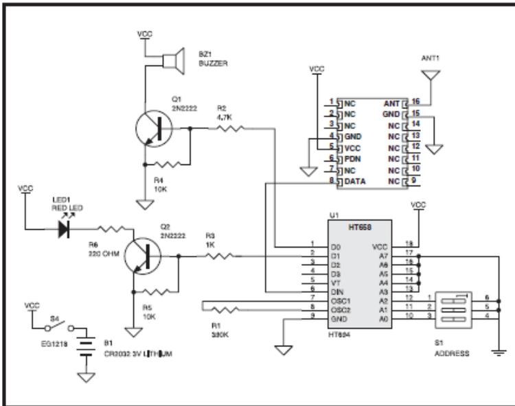
Figure 16: Basic Remote Control Receiver
