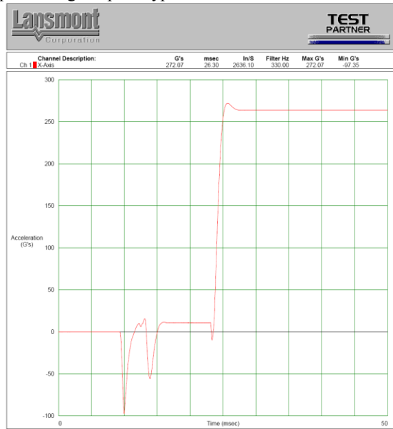
Figure 6: Drop Test Results With Block of Wood
