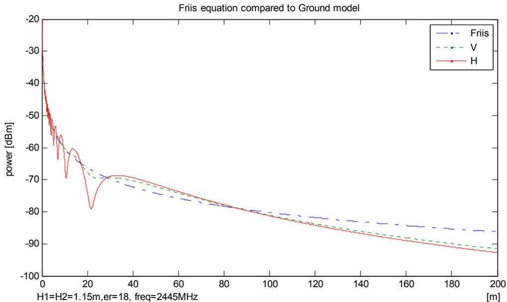
**Figure 2. Difference in Transmission Loss due to Polarization**
